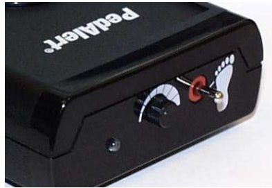
Figure 5. The weight threshold knob adjusts the force required to activate the warning tone.
