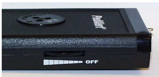
Figure 2. On/Off switch and warning tone volume are set with the same control.
