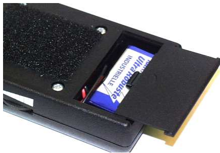
Figure 6. A standard 9V battery is easily replaceable.
